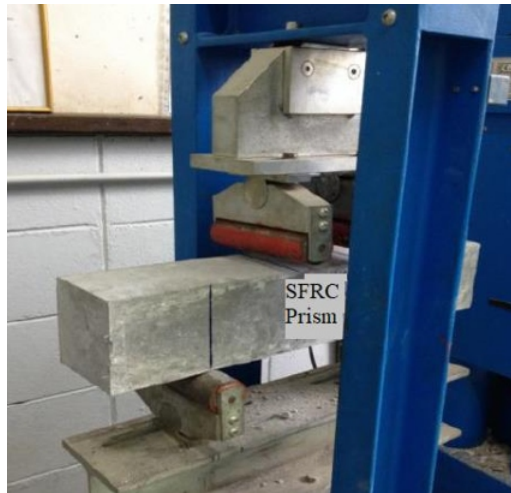
Figure 4. Flexural Strength Test
