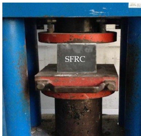
Figure 3. Compressive strength test on Concrete cube samples
