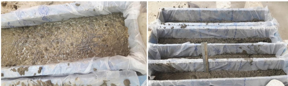
Fig. 2: Layered casting of concrete using steel-brass hybrids.
