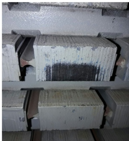
Fig. 4. Molten lump of stator winding coming in contact with slot-tooth, leaving a mark.
