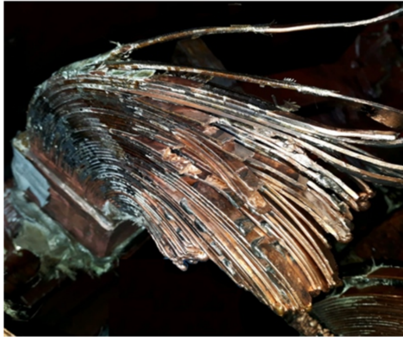
Fig. 6. A damaged coil showing burnt strip conductors in a typical high voltage alternator (Courtesy: Proclaim).
