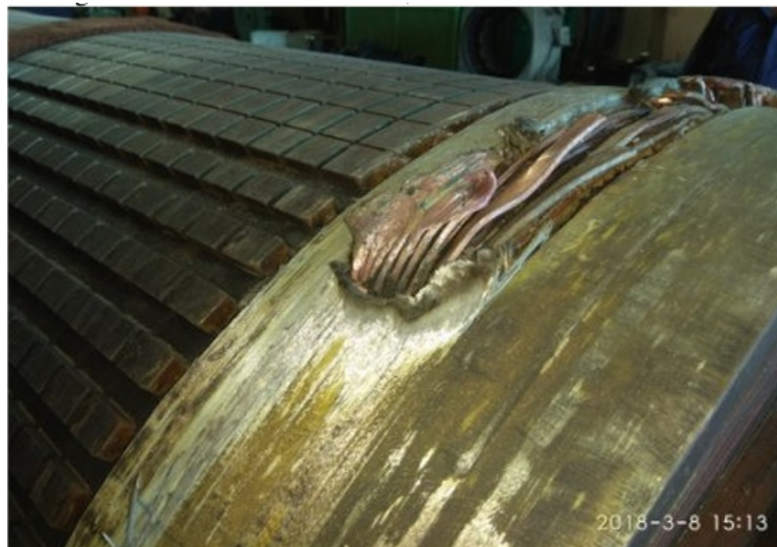
Fig. 8. Puncturing of glass insulation covering the overhang portion of the rotor due to dislocation of stator winding causing direct contact with the rotor.
