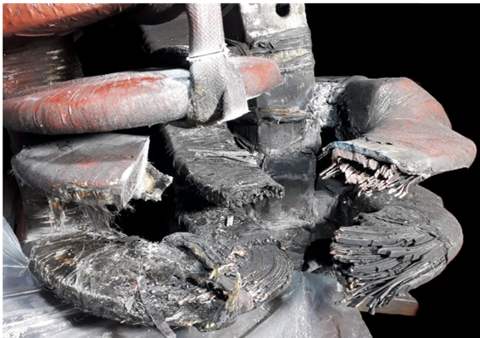
Fig. 9. Nose Joint Failure.
