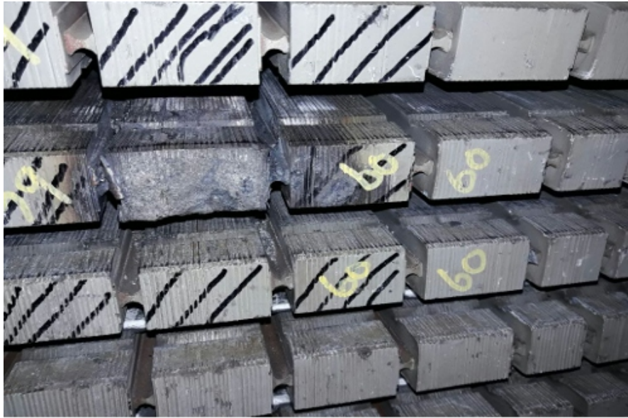
Fig. 3. Burning of packets of tooth stampings in the core.
