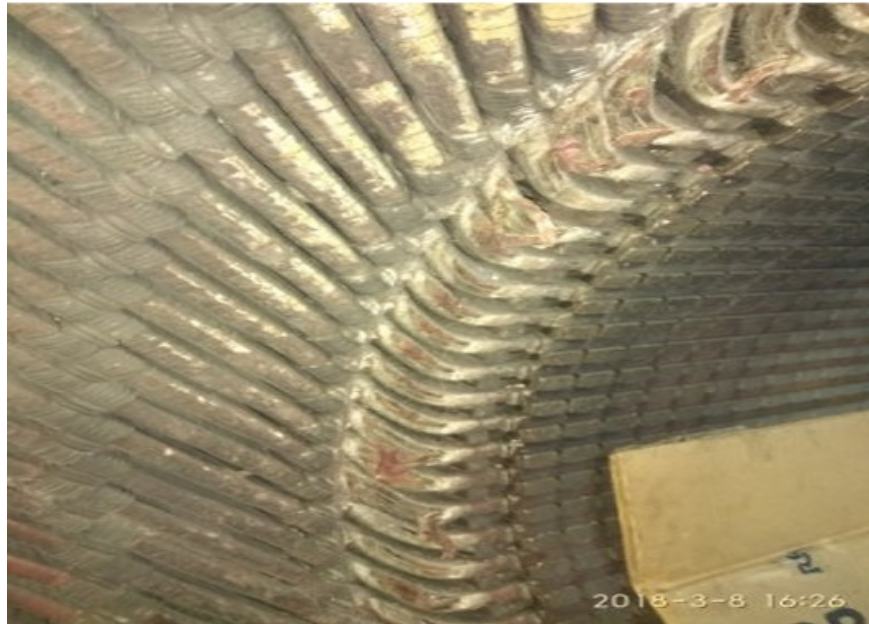
Fig. 7. Deformation of 15 MW, alternator due to dislocation.
