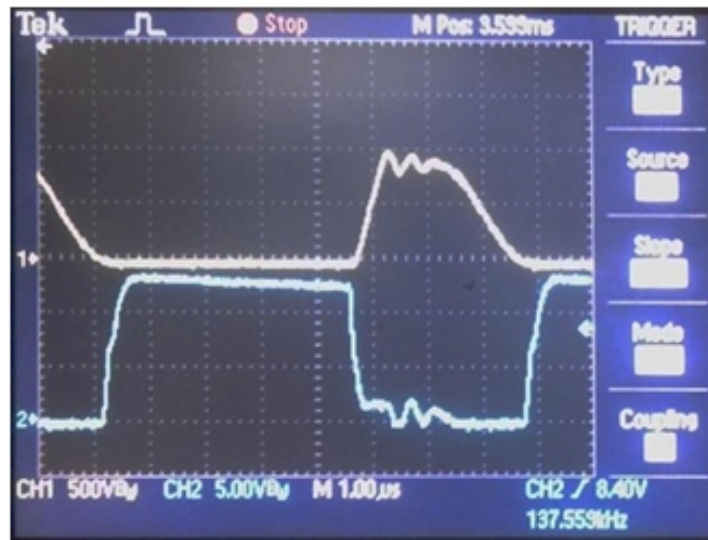
Fig. 4: Gate and Drain full Waveform At 220 V AC input 500W Load
