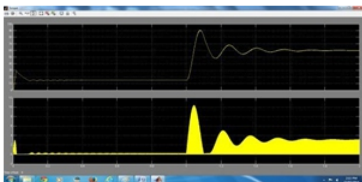
Fig13. Output voltage waveform of boost converter with PWM
