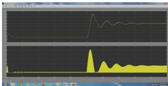
Fig 10. Output voltage waveform of buck converter with PWM
