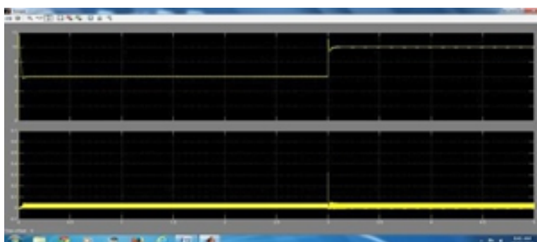
Fig 11. Output voltage waveform of buck converter with PID controller
