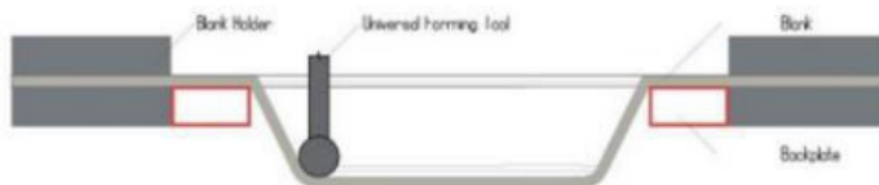
Figure : Single Point Incremental Forming Process
