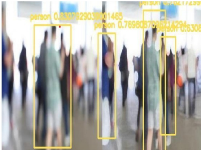
FIGURE3:Applying YOLO to deblurred frame
