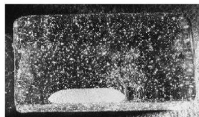
Figure 4: Photograph of bubbles in as-cast glass sample, their thickness are 20 mm [23]
