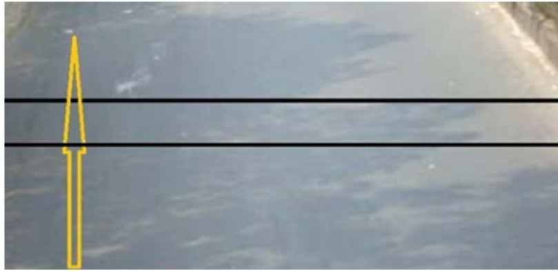
Fig. 4: Two virtual detection lines of a frame. Arrow indicates the flow of traffic and
