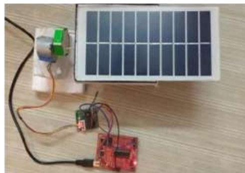
Fig.5 Prototype of a solar tracker system for demonstration
