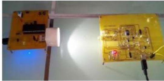
Fig.15. Transmission of signal based on LED lighting.
