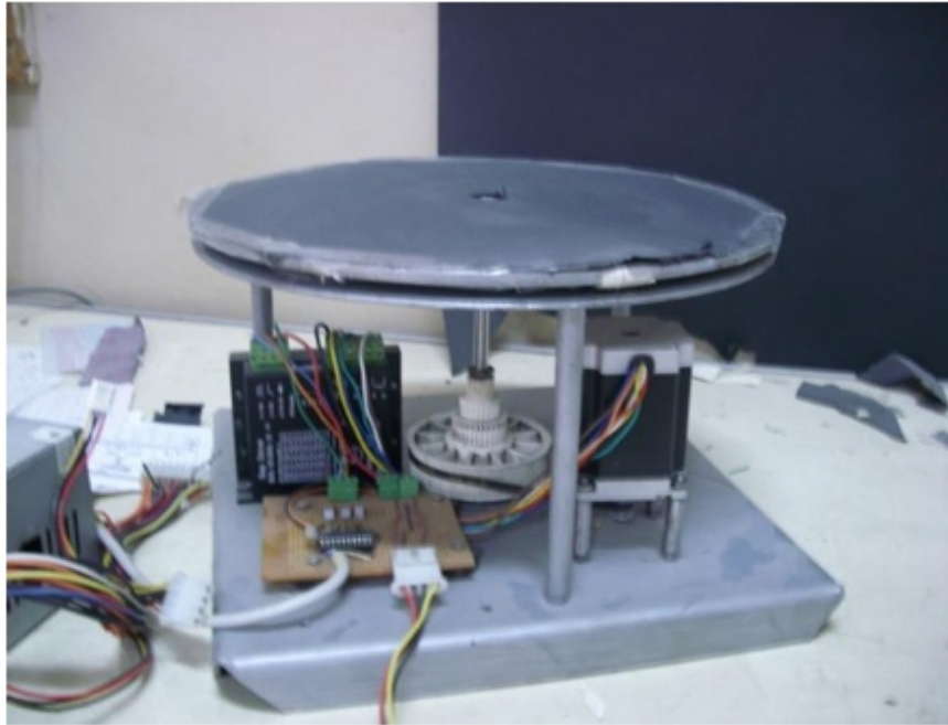
Figure 1. The rotary table is used in our work to change the camera's viewing direction to an object.
