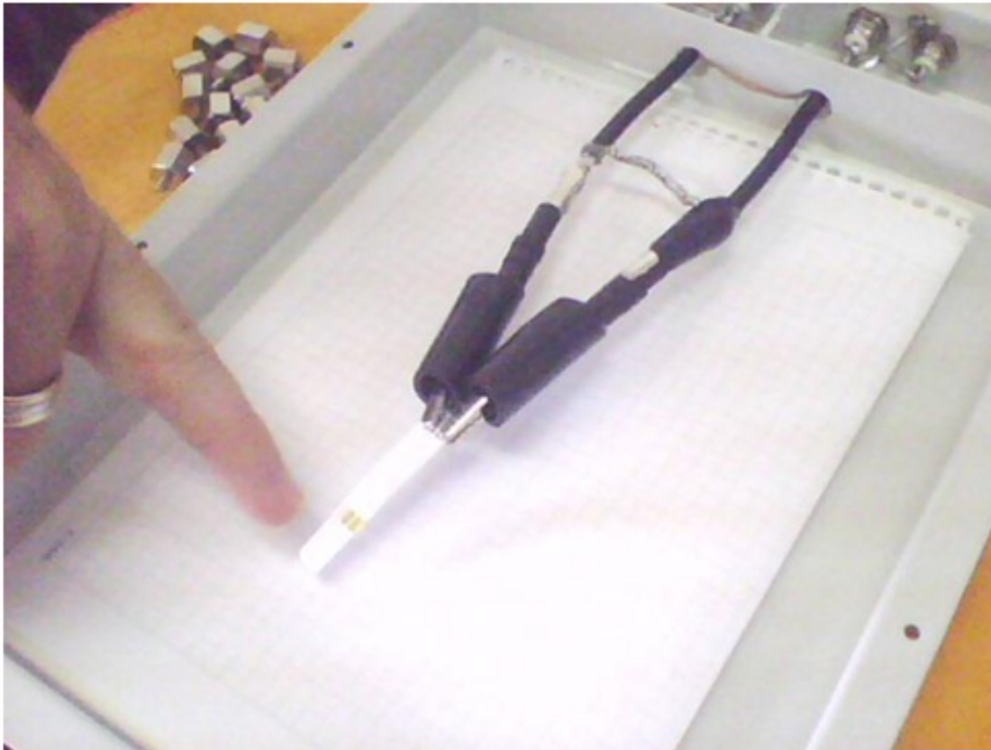
Figure 11 – Biosensor used for the reaction with hemometabolite.
