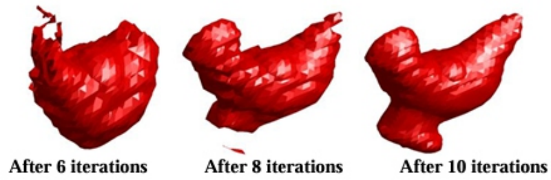
Figure 11. The evolution of the level set function to reconstruct the final surface for the experiment on the 12-frame rooster sequence.
