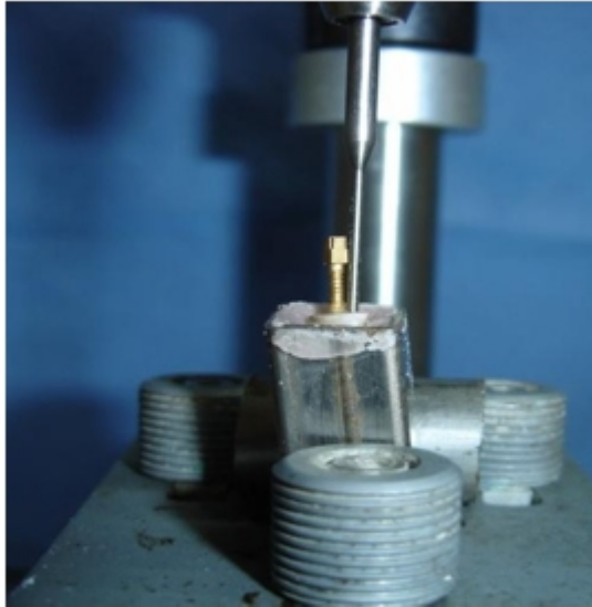
FIG 1: Mounting the specimens with a surveyor to ensure parallelism
