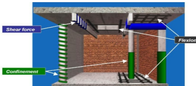
Figure 4 . Different kinds of carbon fiber strengthening (AmélieGrésille 2009)
