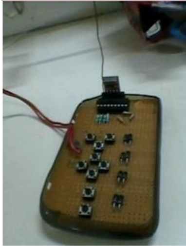
Figure 6: Remote to control the functionalities of IMGROB robot
