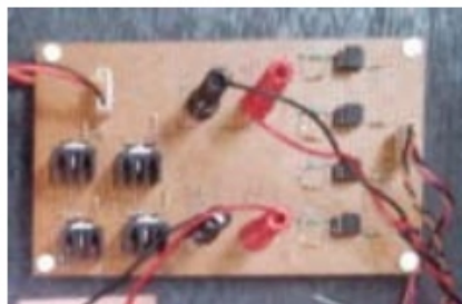
Figure 3: Connections of MOSFETs with battery and motor
