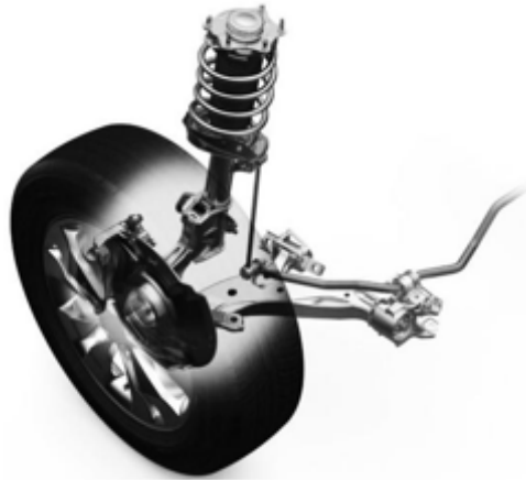
Figure 1: A unit view of a suspension system
