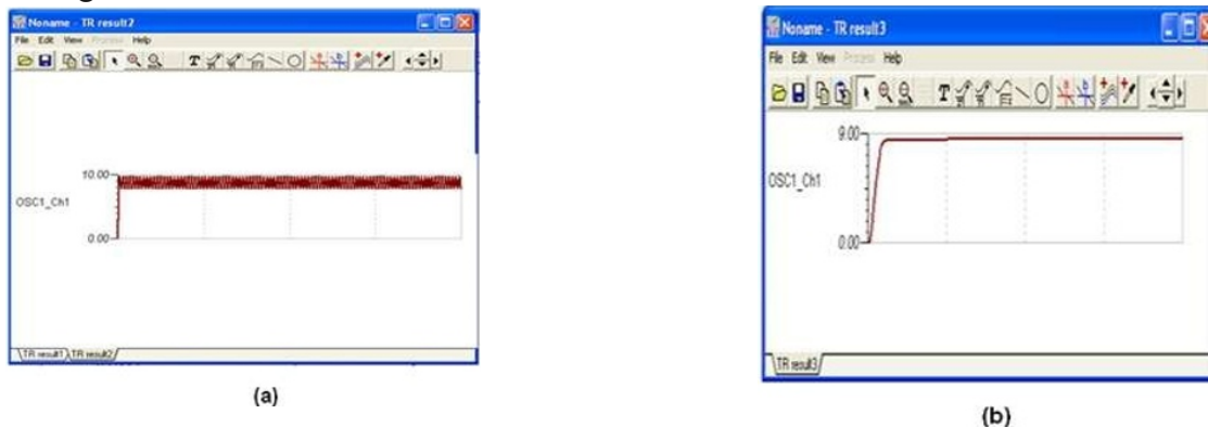
Figure 6.2: Output voltage obtained using circuit used by Guan's circuit (a) and used by Ottman's circuit (b)
