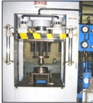
Fig. 2 Experimental setup on 100 tonne double action hydraulic press
