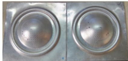
Fig. 3 LDH tested specimens showing biaxial stretch
