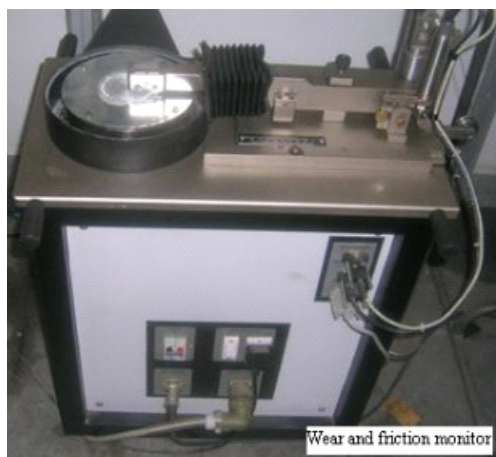
Figure 1: Friction Monitor Used for the Friction Tests
