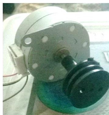
Figure 12. Stepper motor with mounted pulley and wiring to measure V-
