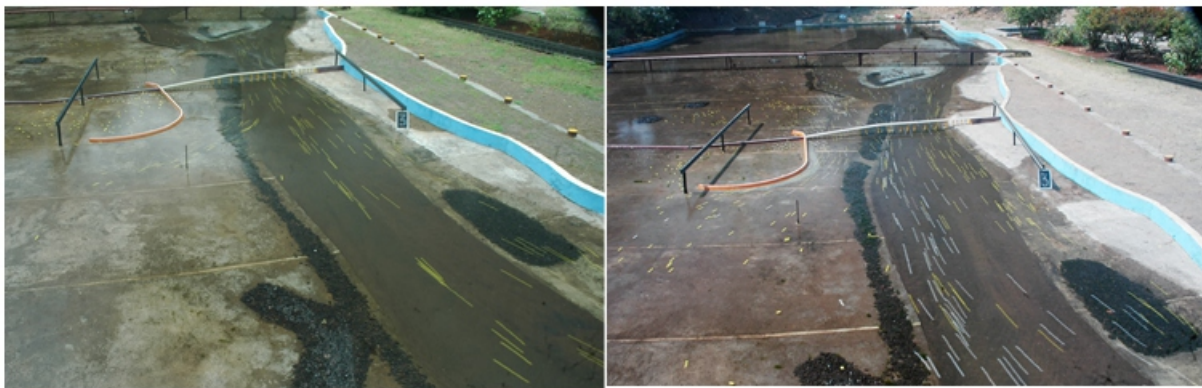
Photo3 Flow conditions with original alignment of Guide bund
