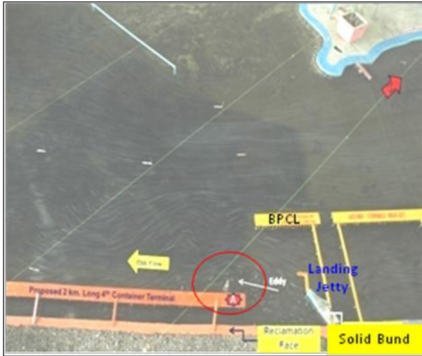
Figure 9(a) Eddy at north end due to solid Bund
