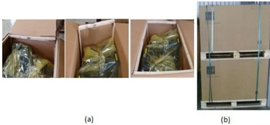
Figure 2 (a) Engine packaging in wooden cardboard box (b) The old packaging methods with wooden pallet and card board box packing inside the containers with nylon taps
