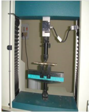
Figure-3. Beam of Material Under Bending
