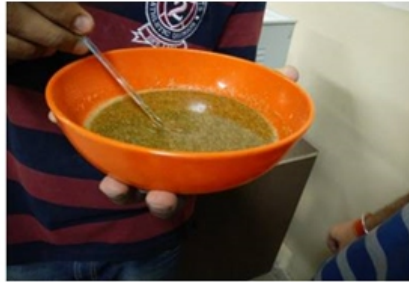
Figure 6. Mixing of Epoxy resin and Sugarcane Trash
