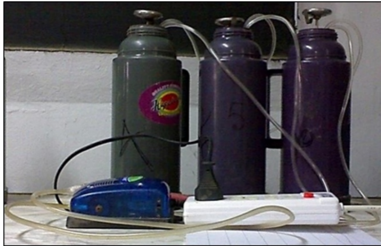
Fig. 2: Experimental Setup for Temperature Variation during Forced Aeration Composting.
