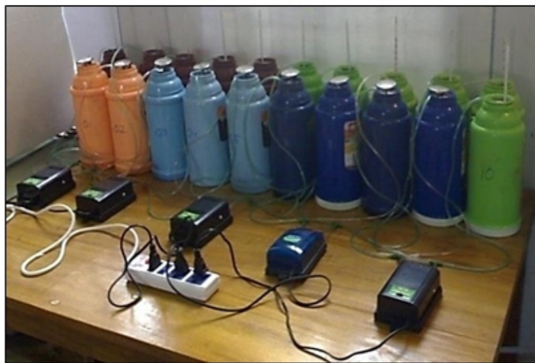
Fig. 3: Experimental Setup for Determination of Volatile Solids Degradation.
