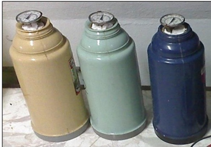
Fig. 1: Experimental Setup for Temperature Variation during Passive Aeration Composting.
