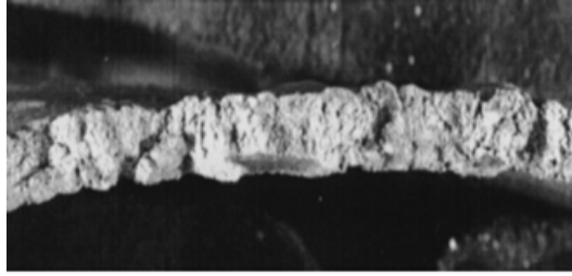
Fig.2 Macroscopic Picture of Cracked Weld Joint (Source: A. Adamkowski-2001)
