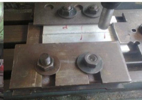
Fig. 3.1.5: Fixture setup on milling machine
