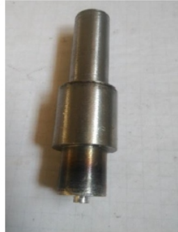
Figure: 3.2.1 FSW circular pin profile
