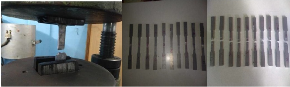
Figure: 3.3.2.4: Testing of Specimen in UTM Figure: 3.3.2.5(a & b): specimen before & after testing
