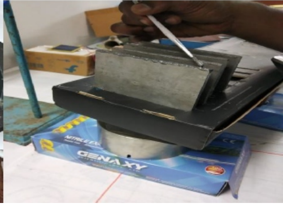
Figure: 3.1.2 Coating of the magnesium slurry on the base metal
