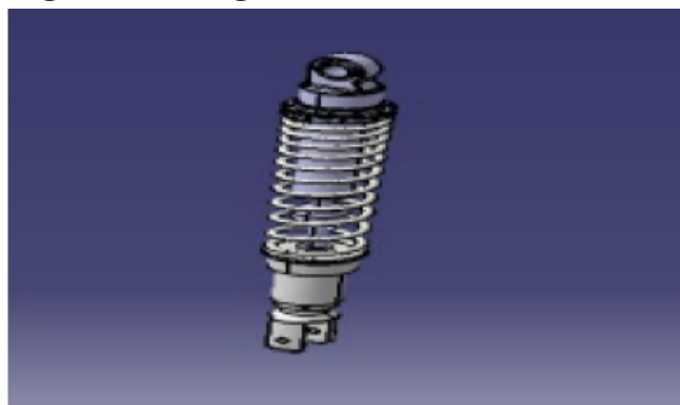
Figure: Modified shock absorber total assembly
