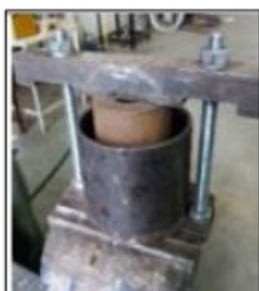
Figure 2. Mold with composite material during the pressing process
