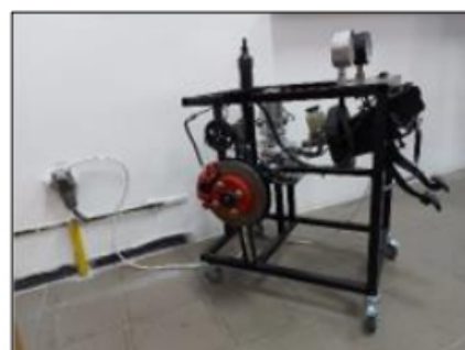
Figure 6. Experimental installation for intensive braking
