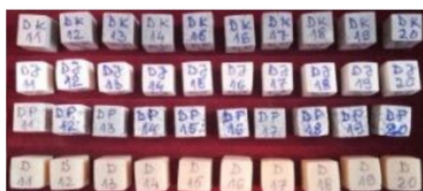
Figure 1. Specimens of specimens for compression stress with matrix based on Dammar
