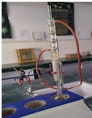
Figure 4. Assembly set for extraction of eucalyptus extracts
