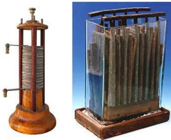
(a) The Voltaic battery (b) Gaston Planté's battery.
