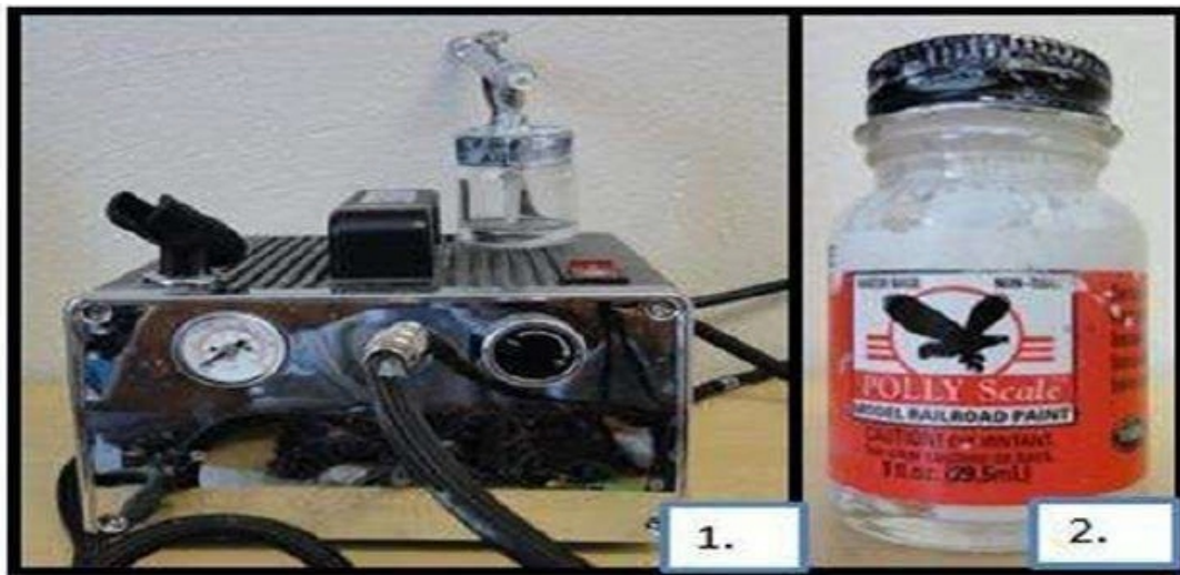
Figure 4.5.1.1 Spray paint gun and air pump, (2) Polly Scale white paint water base
