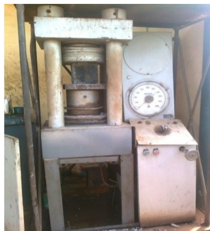
Figure 3. Crushing of a Sample in a Compression Machine
