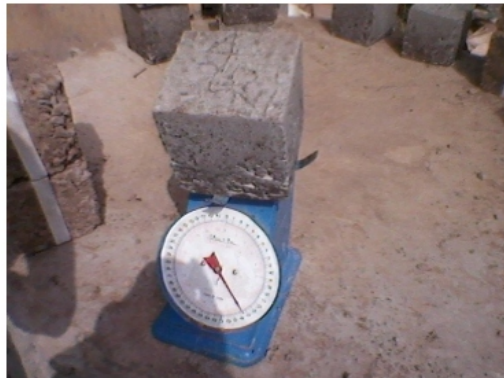
Figure 2. Weighting of a cube sample
