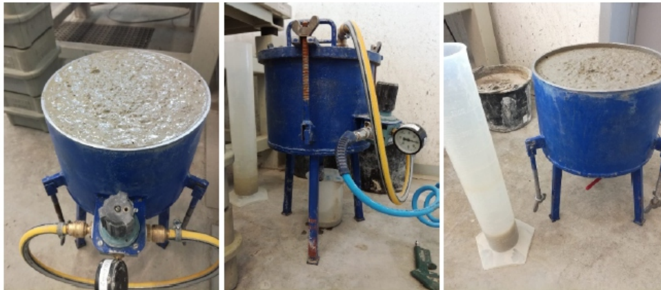
Figure 5. Equipment for determining water separation from concrete according to ÖBV during and after the test
