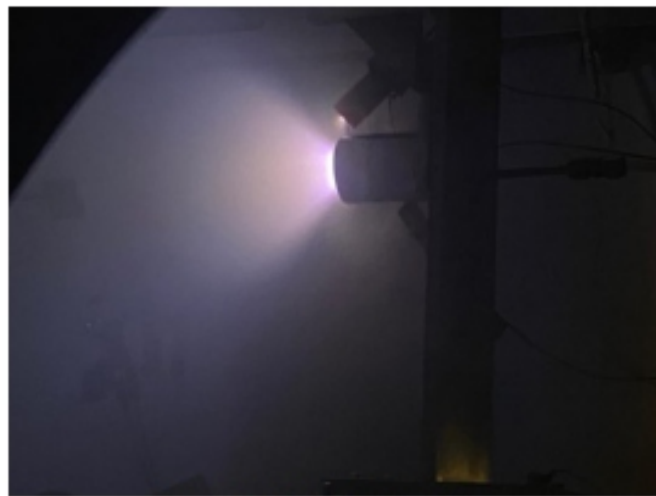
Figure 5. Picture of CFHT-27 in operation inside the vacuum chamber.
