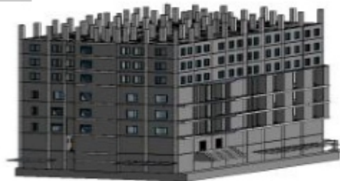
Figure 29: 7th floor level beam Figure 30: 8th floor level and slab, 5th FL wall and floor and column and 7th floor level stair and 4th FL D & W for phase 19 shear wall, 6th floor level wall and floor and stair and 5th FL doors and windows for phase 20
