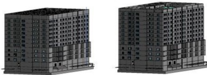
Figure 39: 12th top FL beam Figure 40: 13th roof level and slab, 11th FL wall and floor column and 12th top floor and stair and 10th FL D & W for phase 29 level shear wall, top floor level wall and floor and stair and 11th FL doors and windows for phase 30
