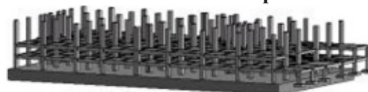
Figure 16: 1st floor level column and ground level shear wall for phase 6
