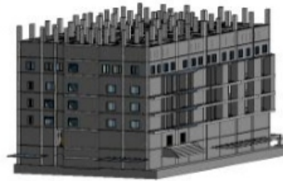
Figure 27: 6th floor level beam Figure 28: 7th floor level and slab, 4th FL wall and floor and column and 6th floor level stair and 3rd FL D & W for phase 17 shear wall, 5th floor level wall and floor and stair and 4th FL doors and windows for phase 18
