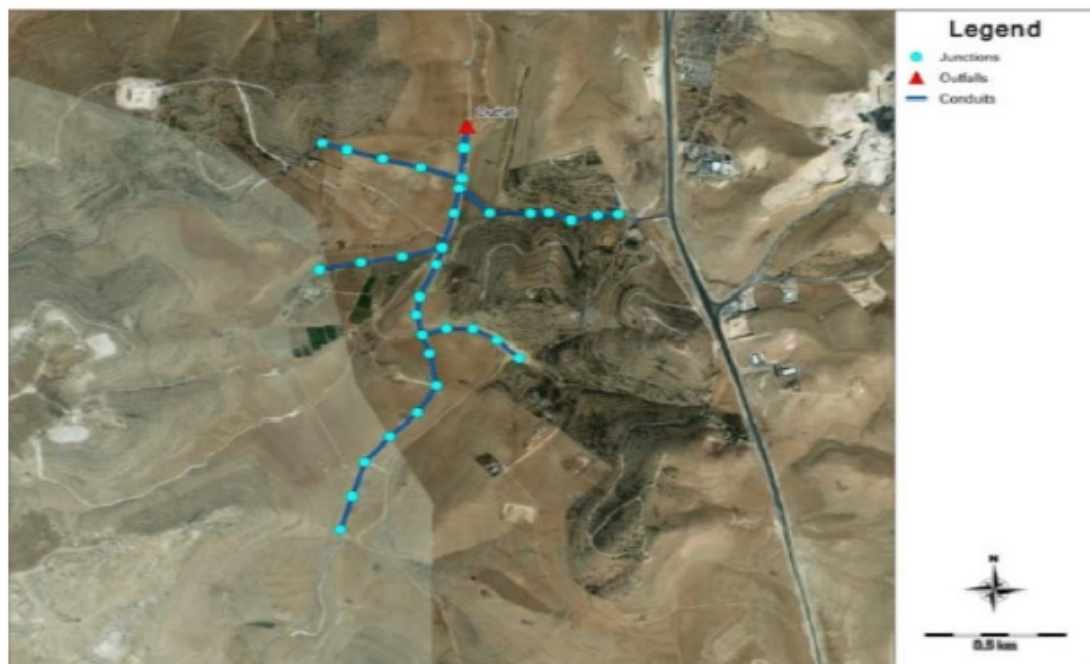
Fig. 3. Pipe network layout
