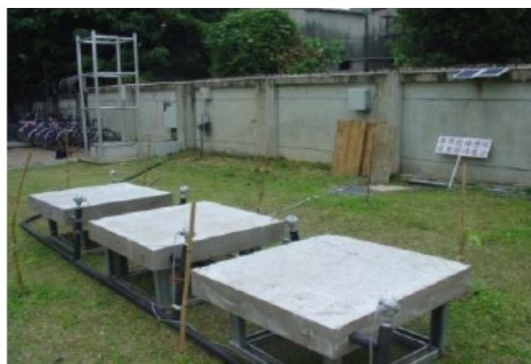
Fig. 1 Installation of the pilot testing concrete wall plate
