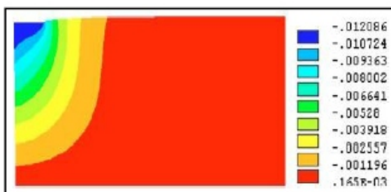
Fig.6 Displacement contours with UDA (M20 joint, L=40 m)
