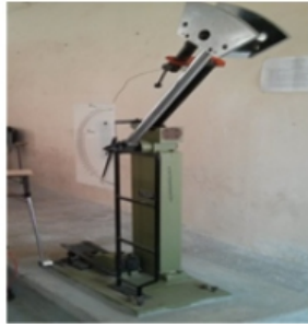
Fig. 8 Impact Testing Machine & its Specifications
