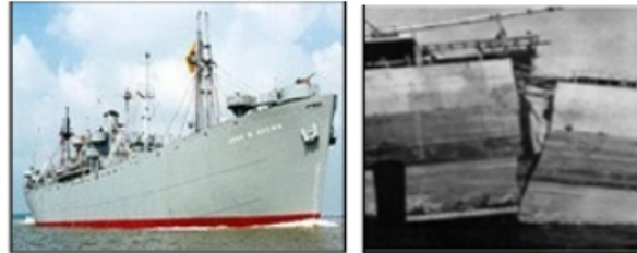
Fig.1 Liberty Ship & Brittle Fracture Seen In Liberty Ship
