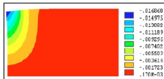
Fig.6 Displacement contours with UDA (M20 joint, L=40 m)
