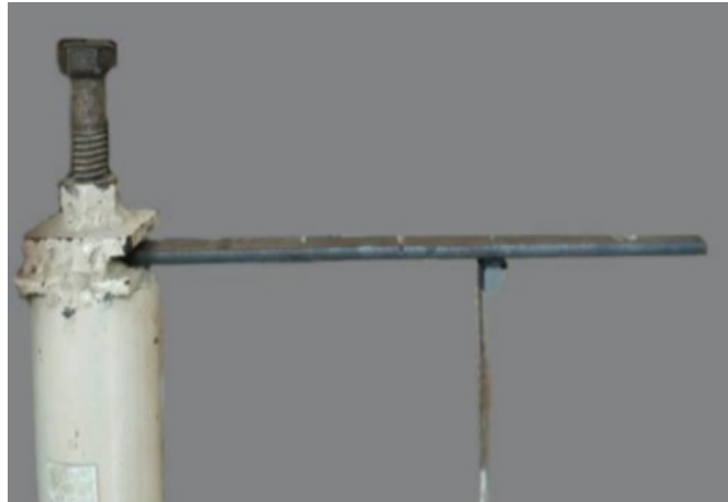
Fig.2. Cantilever beam setup (With an accelerometer and a damage level)
