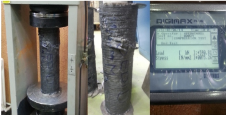
Figure 2. Test set up and shape of failure of circular specimens
