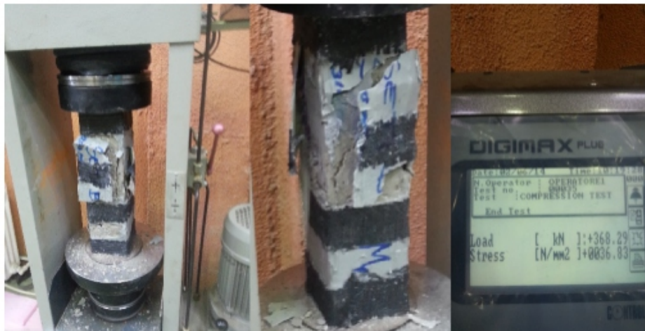
Figure 4. Test set up and shape of failure of rectangular (partially wrapped) specimens
