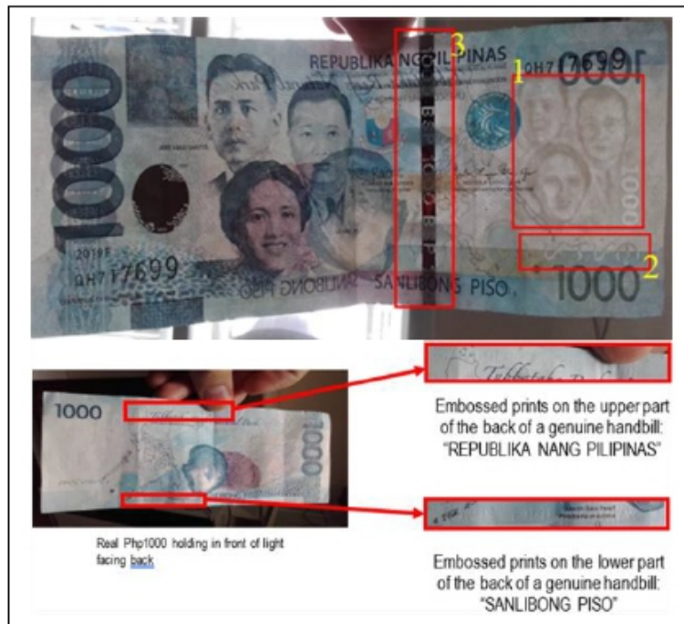
Figure 3. Front (top: 1. Watermark, 2. Baybayin script, and 3. Security thread) and back (bottom) security features of a Philippine peso bill.
