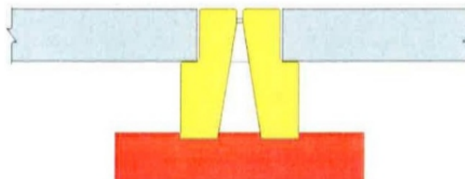
Figure 4: Profile of Original Slot Drain
