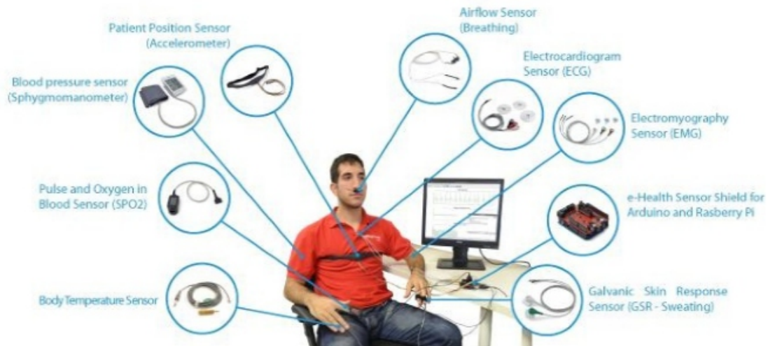
Figure 1: Application of Different types of sensors on human body externally [5]
