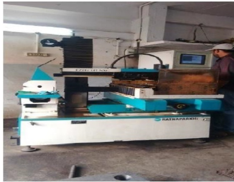
Figure 1. Electronica Ezee Cut Nxg Wedm Machine
