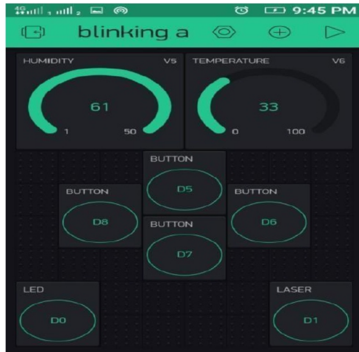
Fig.5. Widget created for controlling Laser shoot, Directional movements, temperature and humidity updates and night vision light by using Blynk.
