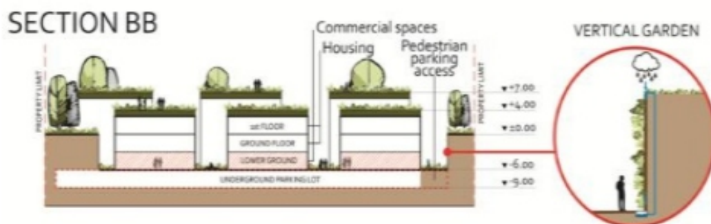
Figure 3 – Complementary functions underground (own contribution)
