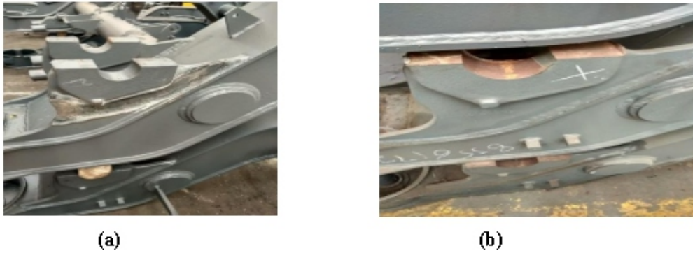
Fig.4 (a) control arm before cutting by machine and(b) control arm with improper depth of cutting
