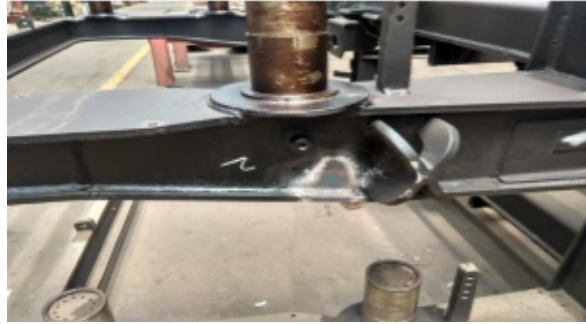
Fig. 8 Distortion in guide of bogie frames
