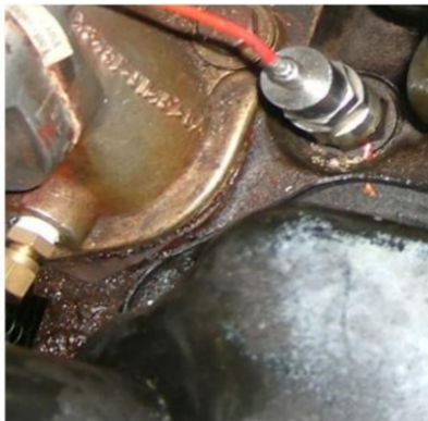
FIGURE 2. VIBRATION ACCELERATOR TYPE 4368 LOCATION
