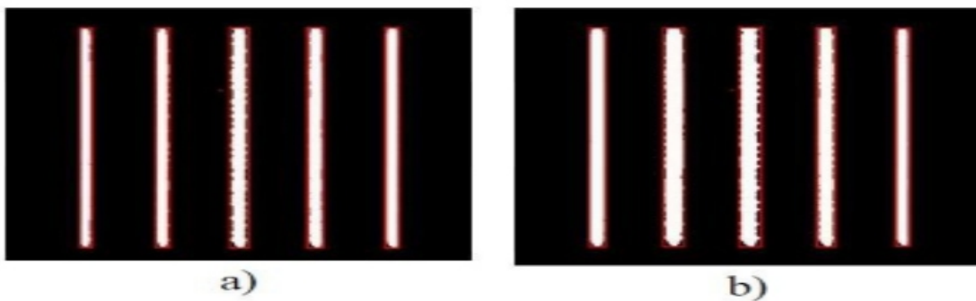
Fig.5. The segmented picket fence: a) The segmented picket fence of static MLC using MATLAB, b) The segmented picket fence of VMAT using MATLAB
