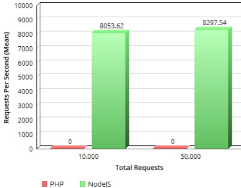
Fig.3. NodeJS and PHP environments, concurrent comparison over 1000 connections
