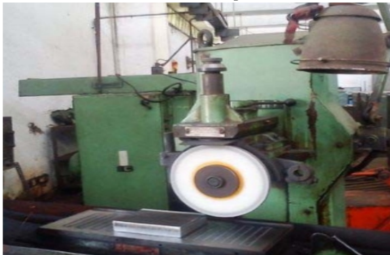
Surface Grinding of H-13
