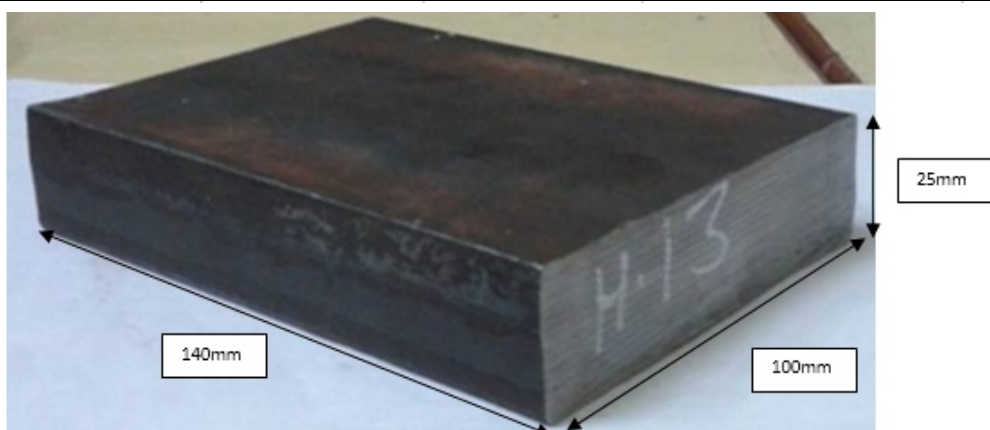
Side view of H-13 material
